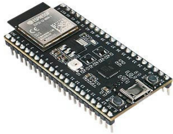
Figure 5: the ESP32-S2 dev board that is used.
