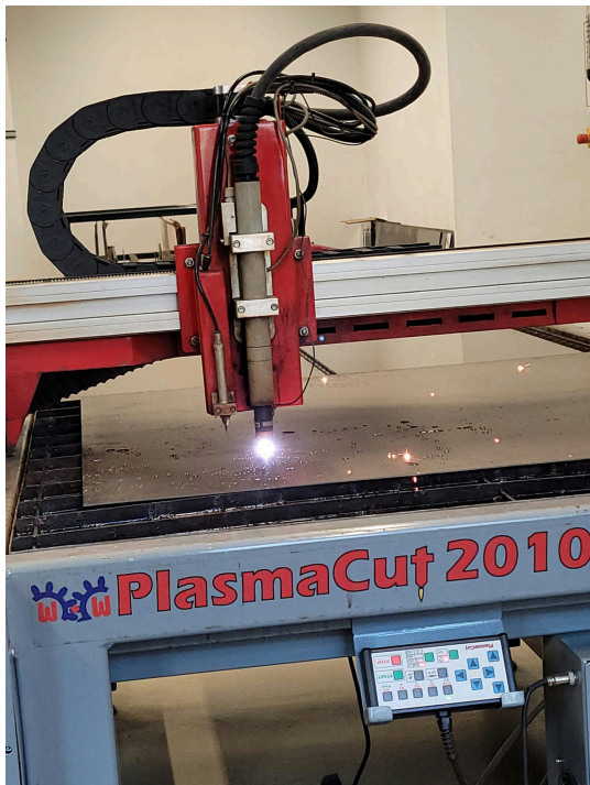
Figure 4: The Plasma cutter in action cutting out the parts.
