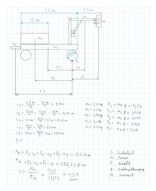
Using the dimensions of the robot, I calculated the distances between the tipping point and the individual parts. I calculated the force for each of the masses. I then calculated the back torque and the tilting torque and calculated the safety. If the back torque were greater than the tilting torque, the robot would tip over and the value for safety would be less than 1. Anything above 1 means that the robot will not tip over. The higher the value, the better.
