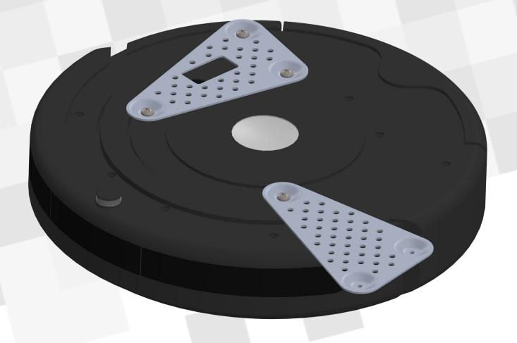
Attach the only the top hole of the other Create bracket to the left side of the Create and rotate it out away from the Create.
