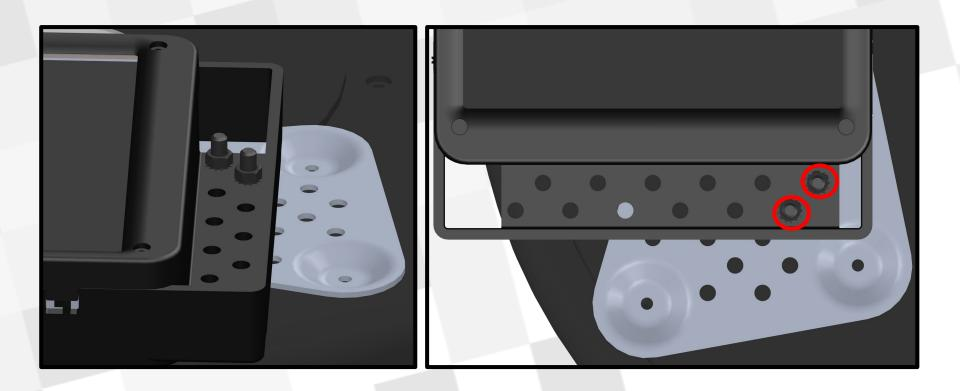
Using to medium bolts attach the Wombat to this Bracket as shown and then rotate the whole piece back towards the Create.
